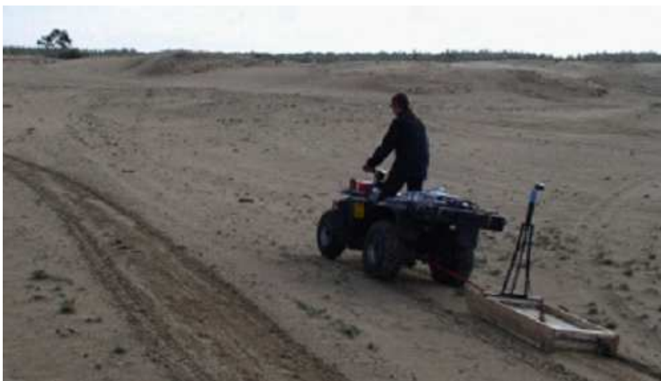
Figuur 43: SP meting. Bron: http://www.medusa-surveys.com/nl/methoden/em_radar/43/groundtracer/
