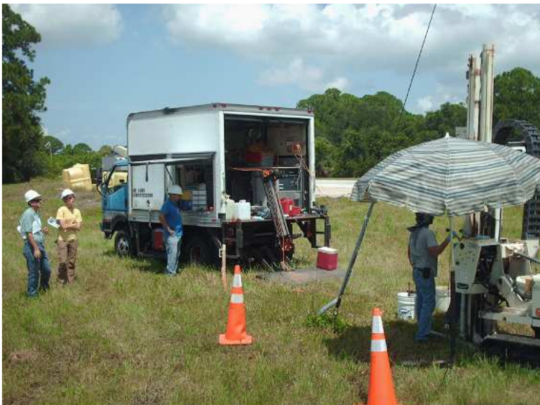
Figuur 37: MIP-CPT. Bron: http://www.kbmobilelabs.com/pages/mip.htm
