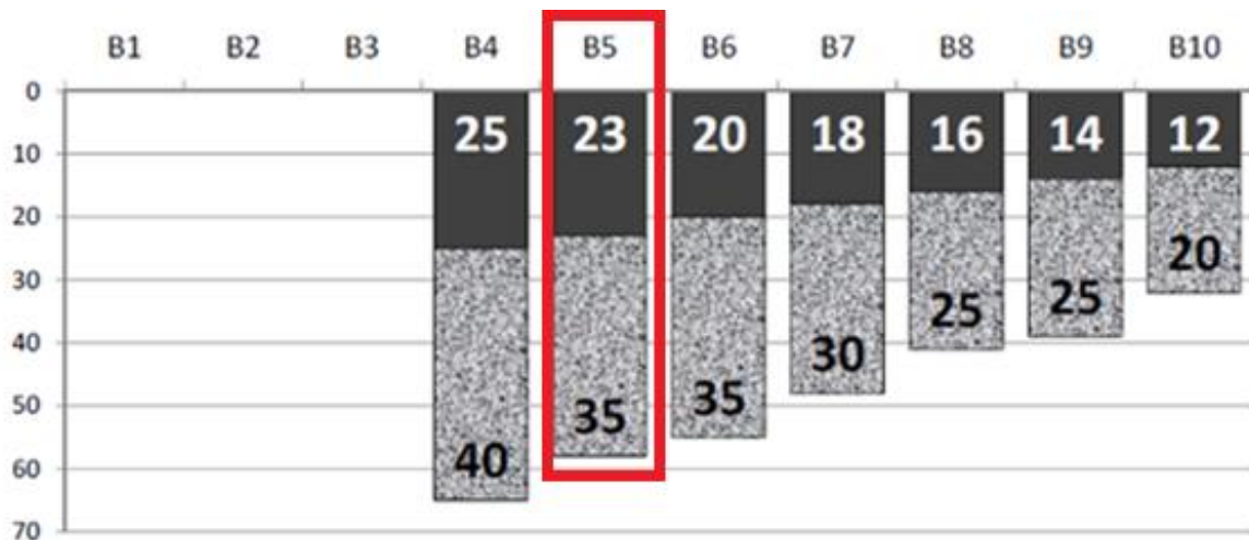
Figure 5: Recommended road structure for bituminous roads in relation to the different traffic classes (following AWW [50])⁴.
