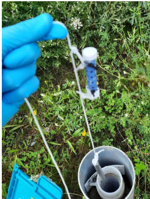
Figure 3 Installation of BACTRAPs at well 8102 (in picture) and 8107.
