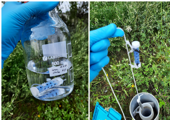
Figure 6: BACTRAP installation in the field in monitoring well
