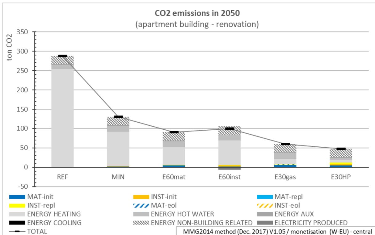
Figure 9. Apartment (1 unit): CO<sub>2</sub> emissions generated over 30 years for different renovation scenarios
