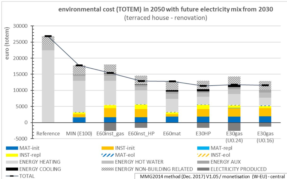
Figure 18. Monetised environmental impact generated by the terraced house over 30 years (from 2020 to 2050) for different renovation scenarios, with future electricity mix after 10 years
