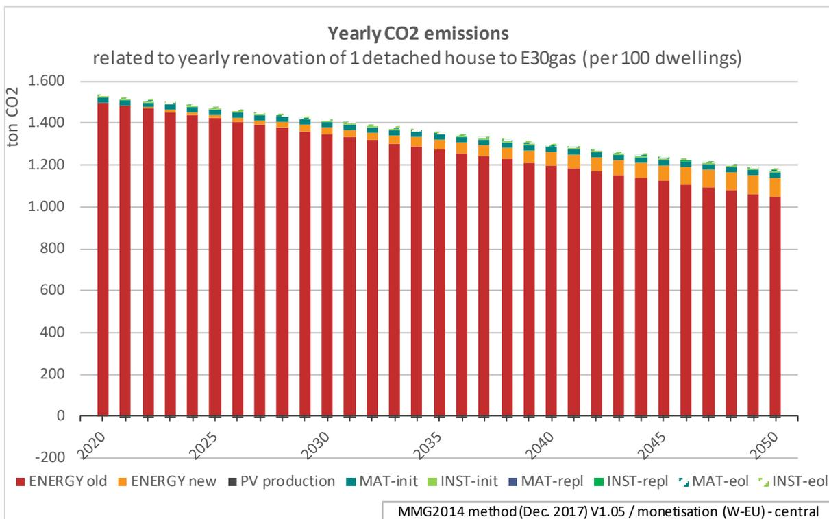
Figure 20. Yearly CO<sub>2</sub> emissions related to a set of 100 detached buildings, considering the renovation of one house each year (1% renovation rate) according to the E30gas renovation scenario
