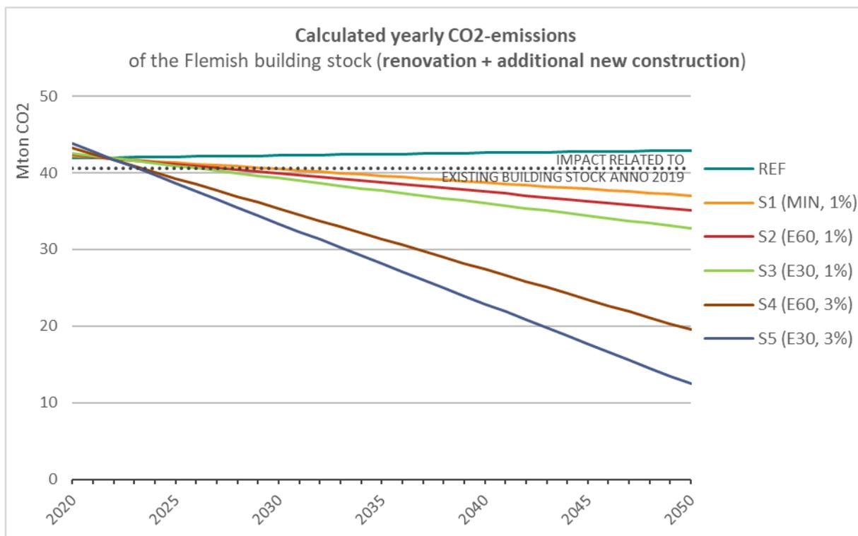
Figure 24. Calculated yearly CO<sub>2</sub> emissions related to the Flemish building stock in case of different renovation scenarios, including additional new construction each year of 20.000 housing units.
