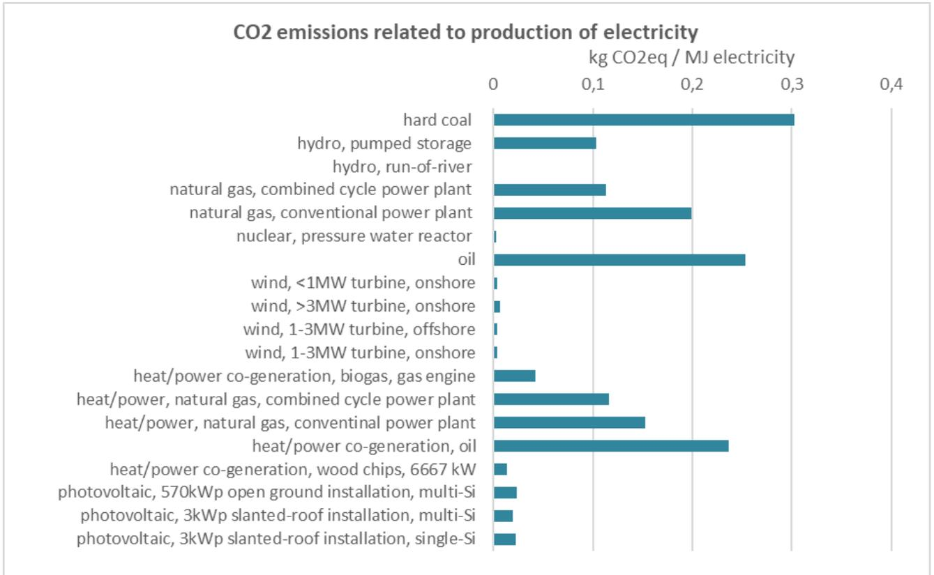
Figure 15. CO2 emissions related to the production of 1 MJ electricity produced by different power plants.
