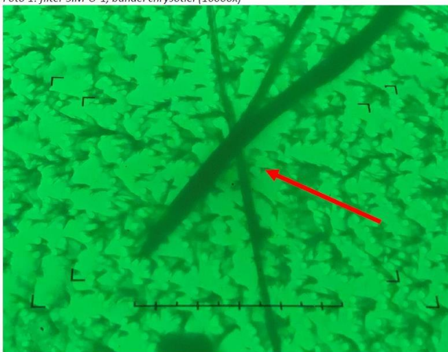
Foto 1: filter SIM-O-1, bundel chrysotiel (10000x)
